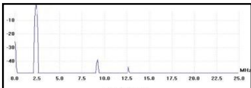
AZ-58 without ray tube at 2,400,000 Hertz measured with spectrum analyzer showing no real harmonics.
